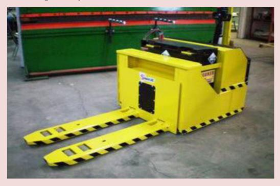
The main function of an electric walk-behind pallet truck is to thoroughly displace and store heavy amounts of goods and pallets from one location within the premises of the facility. Since these are driven by powerful electric motors, these trucks can handle various loads thoroughly while reducing the physical strain on the people working there. They also speed up the transportation process, which multiplies productivity.
